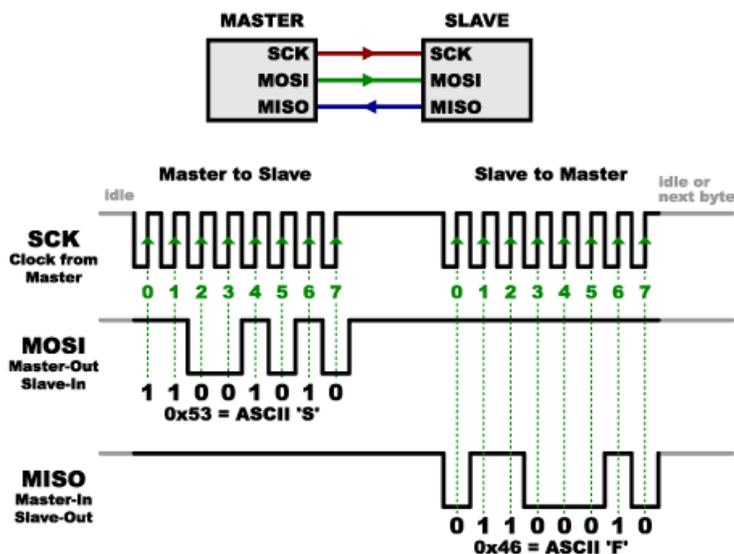
In our project, we have configured a master and only a slave - the DAC module. Data is sent to the microcontroller as a string, is decoded and transmitted to the digital - analog converter; in this way, an increasing or decreasing V out value will result in a sine wave.
