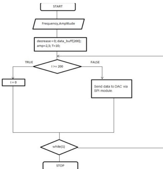
The main idea is to control the frequency and the amplitude for the signal to be via USART from PC to microcontroller. The connection between XMC1100 and DAC (MCP4921) module is made through the SPI communication interface. The output of DAC,  $V_{out}$ , will be watched on the oscilloscope.
