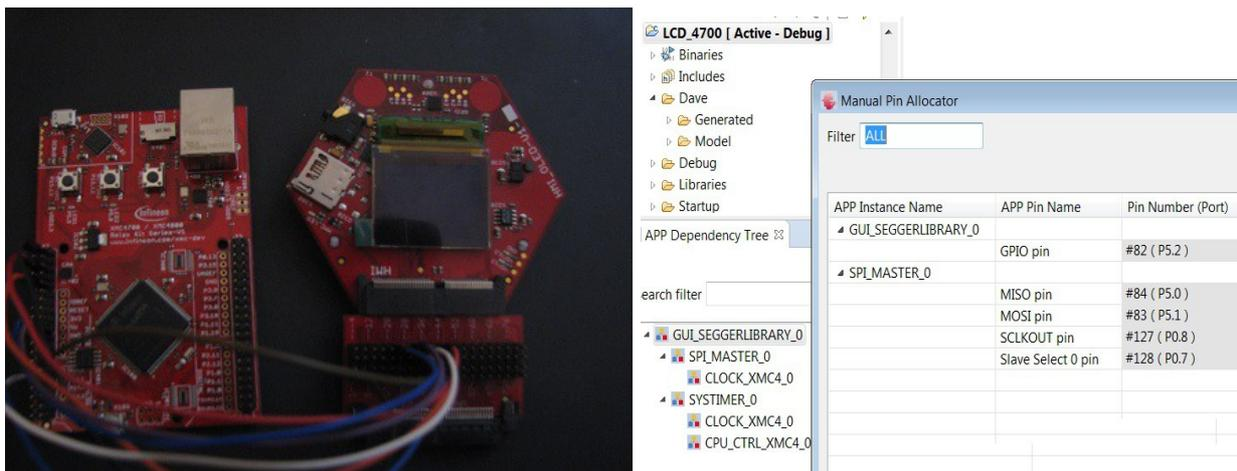
Initially, we connected all the hardware used with the development board and made the software settings to use the functions of the Segger emWin5 library. We have upgraded the GUI.h paths in prj-properties according to the GUI\_Zagger\_lib help specification and set the speed to 1000 and SPI mode with uplinked synchronization.
