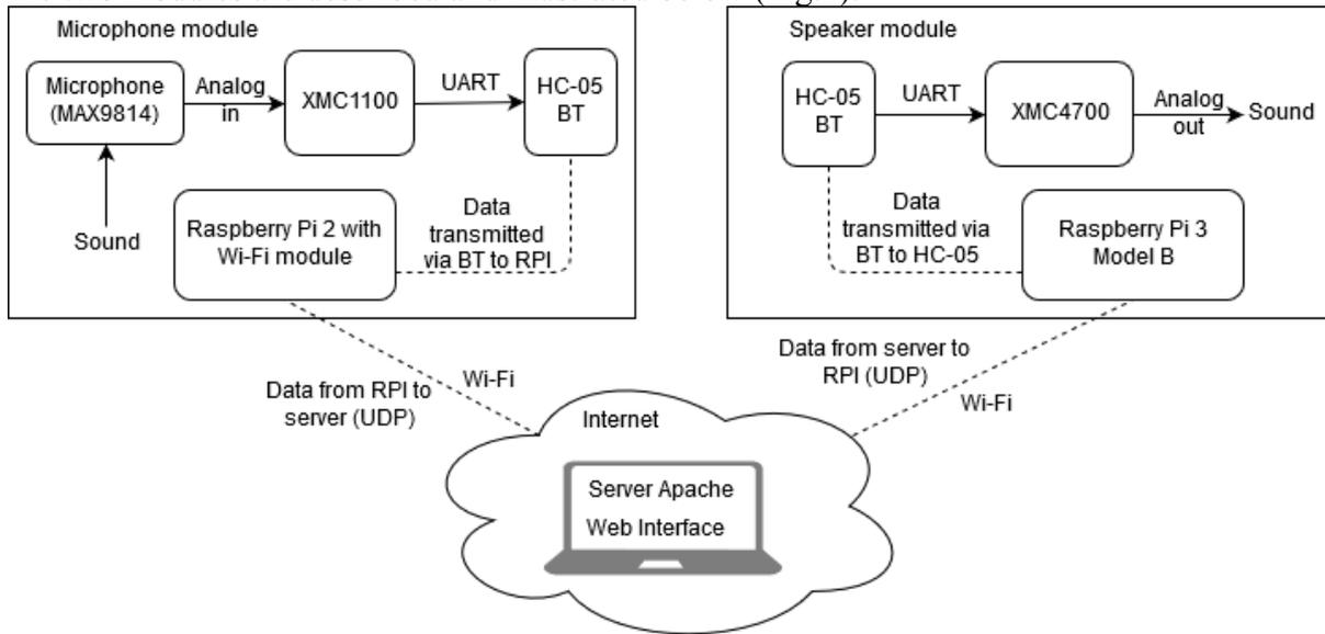
Fig.2 Module components and their interaction
