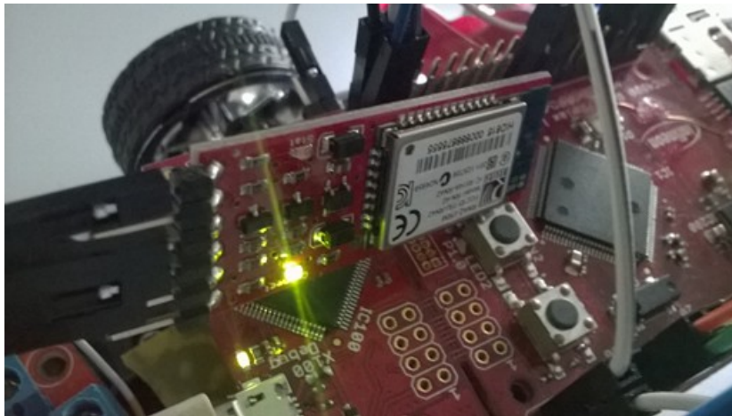
Figure 4 The Bluetooth module
