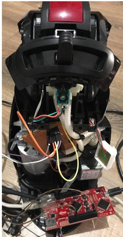
Figure 1 Remote operated coffee machine
