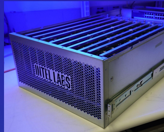
Pohoiki Springs system with 768 Loihi chips
