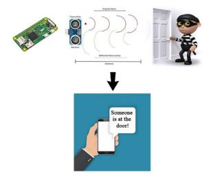
Story: This is a system that uses an ultrasonic sensor to detect if there is an obstacle at a distance of less than 25cm from it. In case there is an obstacle (possible intruder), it sends a signal to a buzzer that starts ringing and also sends an email to a predefined address.
